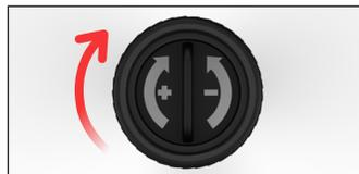
6. Fasten the disc inside the handle (turn to +). If necessary, press in on the opposite side.
