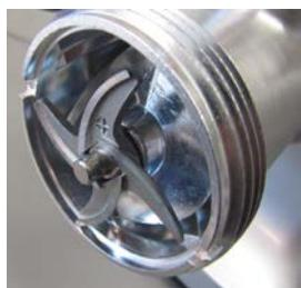
e) Place the cutting plate (10, 11 or 15) on blade (9) and snake (8)
