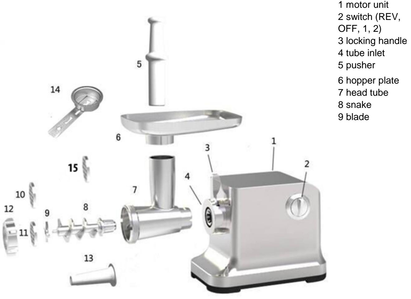
10 cutting plate medium (5mm)    11 cutting plate coarse (8 mm)    15 cutting plate fine (3 mm)
